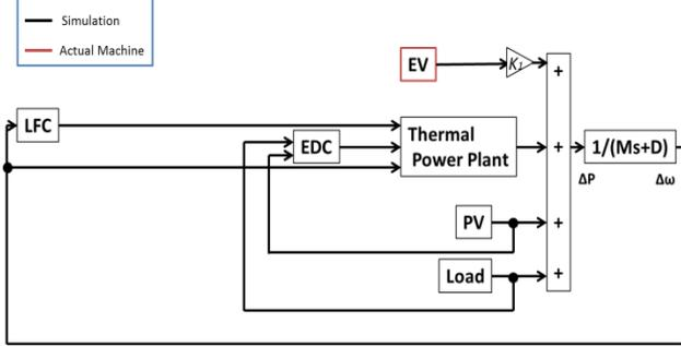
Figure.1 Power system model
