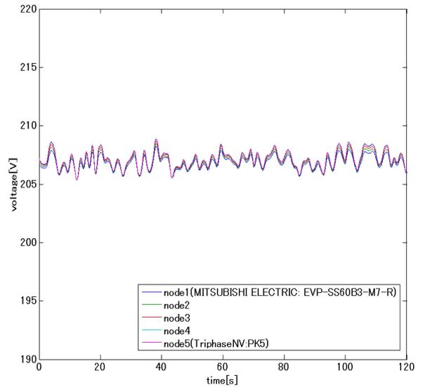
Figure.11 Simulation results of voltage at each node
