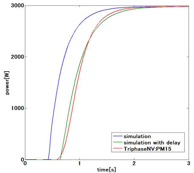
Figure.8 Result of step response test
