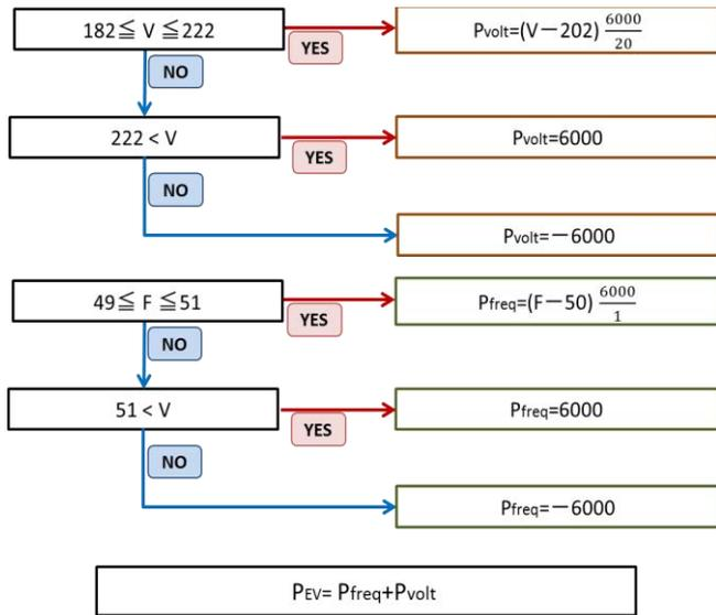
Figure.6 Flowchart of active power control
