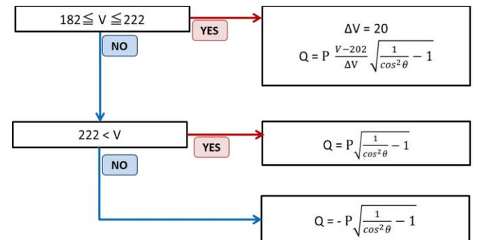
Figure.4 Flowchart of reactive power control
