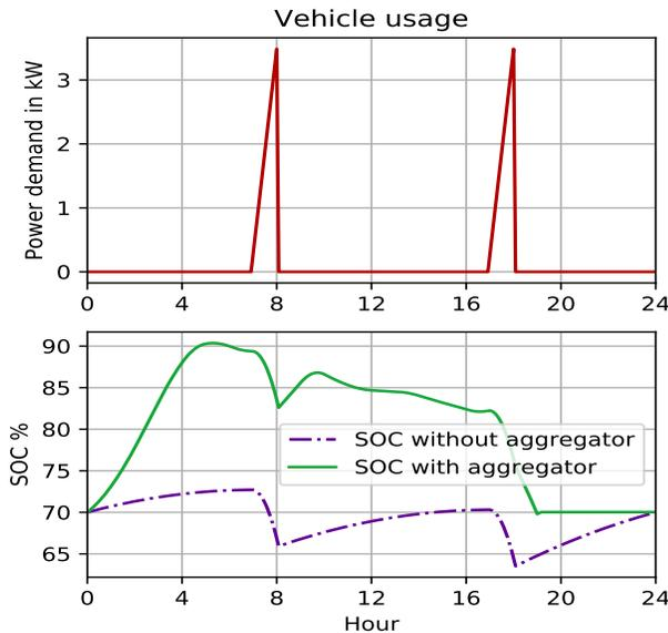
Fig. 14. (a) EV power demand (b) SoC evolution for the most common usage pattern in Bogota
