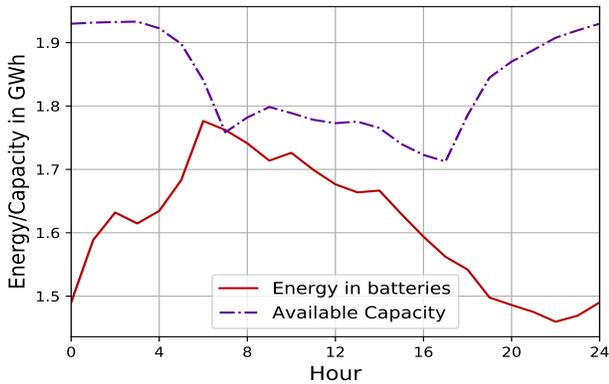
Fig. 10. SoC evolution for the batteries in bus 15
