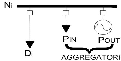
Fig. 2. Representation of aggregators as prosumers in power systems
