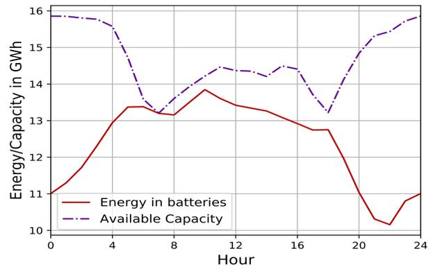
Fig. 12. SoC evolution in the batteries
