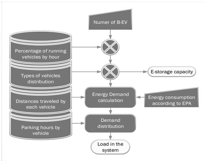
Fig. 1. Methodology for forecast the energy demand of the EVs
