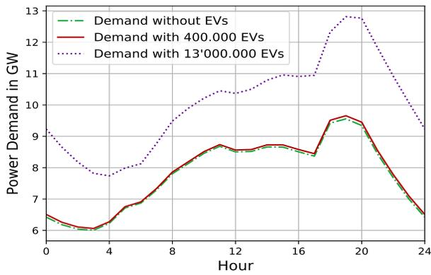
Fig. 5. Comparison between two grades of inclusion of EVs in the colombian case
