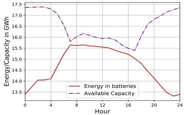
Fig. 8. SoC evolution in the batteries
