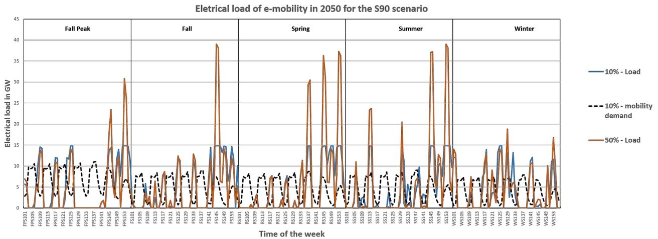
Fig. 10. Electrical load of e-mobility for different charging infrastructure availabilities
