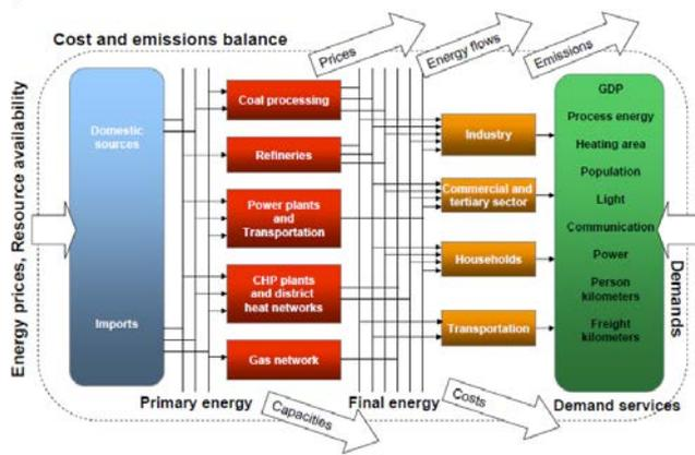
Fig. 1. The TIMES Reference Energy System
