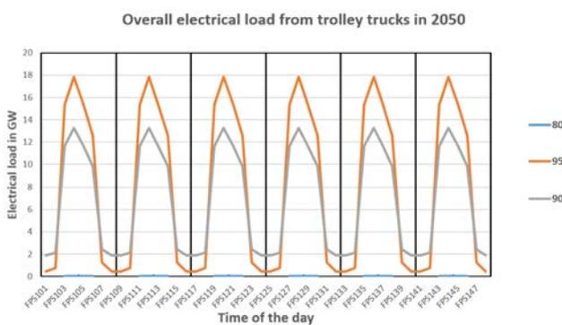
Fig. 7. Load curve of Trolley Trucks in 2050
