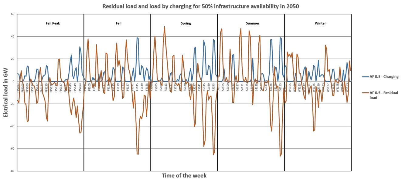
Fig. 12. Residual load and load by charging of e-mobility for 50% infrastructure availability in 2050
