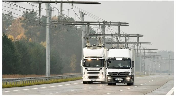
Fig. 2. Trolley trucks on a test track in Germany
