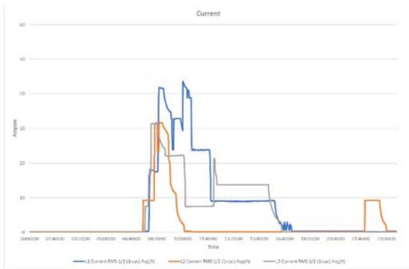
Figure 5 Current at substation A, phase L1(blue), L2(orange) and L3(grey), work day 1
