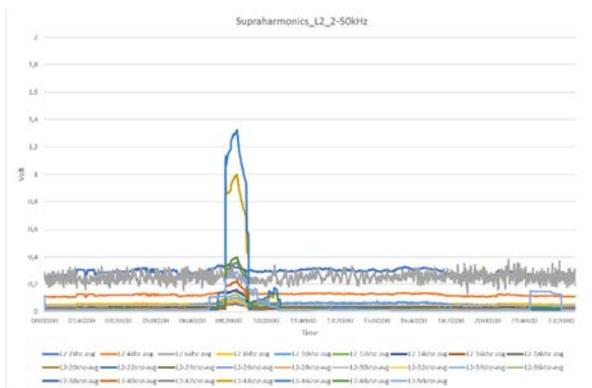
Figure 1 Supra harmonics in phase L2 at Substation A, significant levels of frequency 44 and 46 kHz originated from EV charging, work day 1
