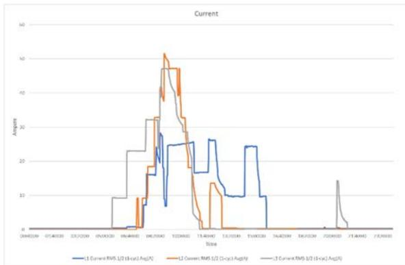
Figure 6 Current at substation A, phase L1(blue), L2(orange) and L3(grey), work day 2
