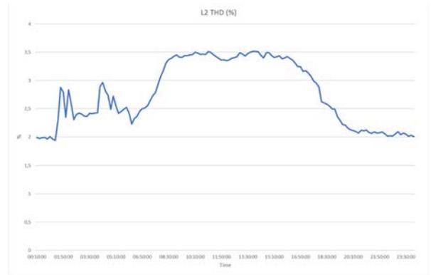
Figure 7 Voltage THD in phase L2 at Substation A, work day 1
