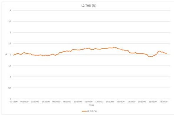
Figure 13 Voltage THD in phase L2 at Substation B, weekend day
