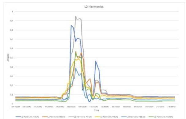
Figure 4 Current harmonics in phase L2 at Substation A, order 3, 5, 7, 9, 11 and 13, work day 2
