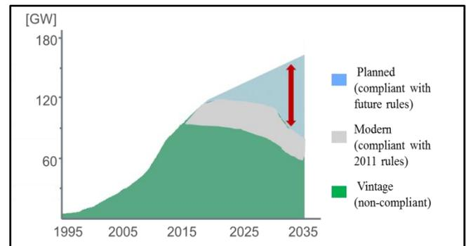
Figure 1. Integration of total VRE systems into the German power grid – approximated figures, adapted from [9]
