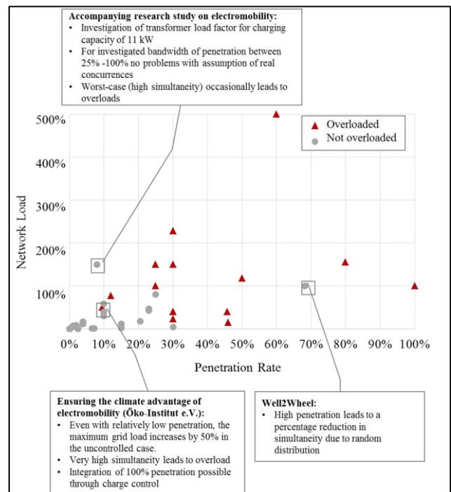
Figure 3. Network load in reference to penetration rate of e-mobility in Germany [7]
