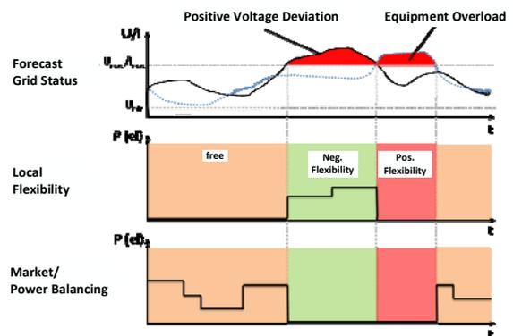
Figure 1 Exemplary control of a PTGP in a critical Situation within the power sector
