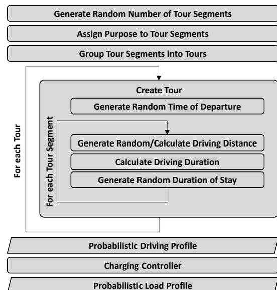
Figure 1: Simulation algorithm for generating probabilistic driving and load profiles
