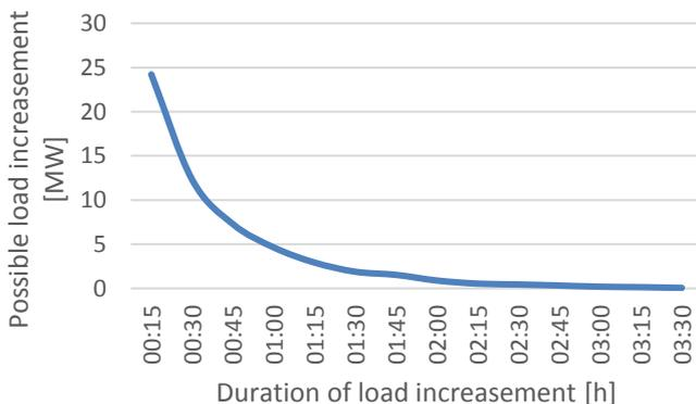
Figure 4: Load increase potential of the EV pool
