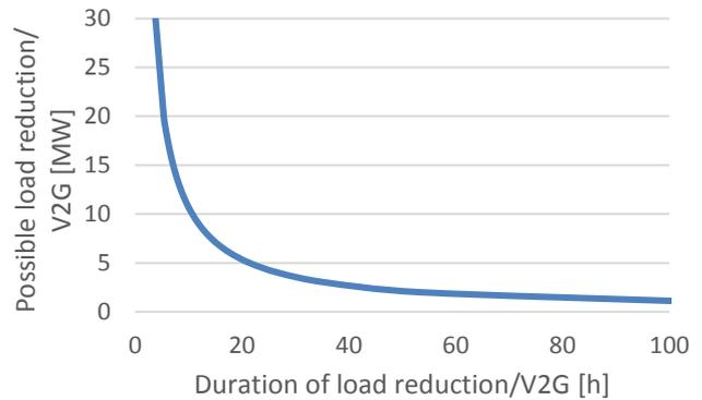
Figure 5: Load reduction resp. vehicle to grid (V2G) potential of the EV pool
