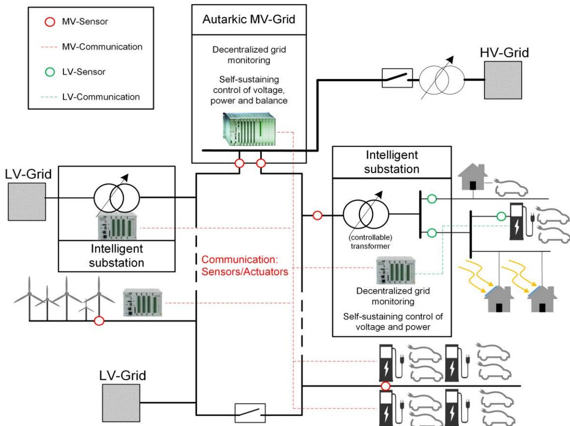
Figure 3: Concept of an autarkic control system on the medium voltage level
