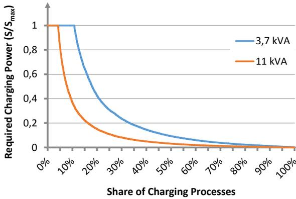
Figure 2: Required charging power for EVs without limiting the users' mobility
