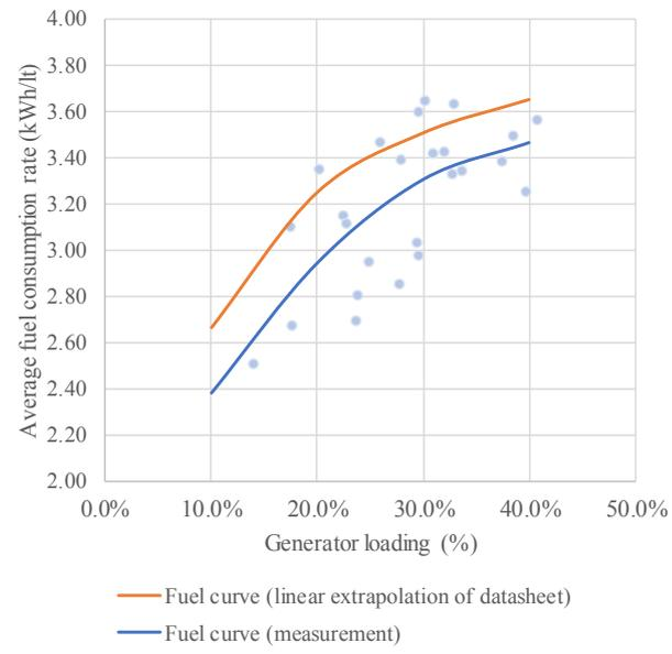
Figure 2. Specific production of a 400 kW diesel generator set operated at low loading
