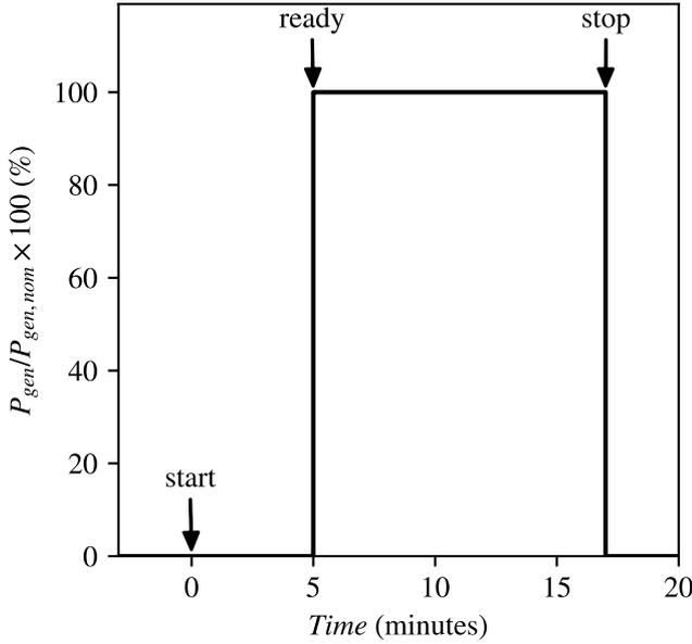
Fig. 1. Illustration of the functioning process of the modelled gensets. The gensets are (ready) delivering their output power 5 minutes after they have been ignited (start) and can be switched off instantaneously at any given time (stop).
