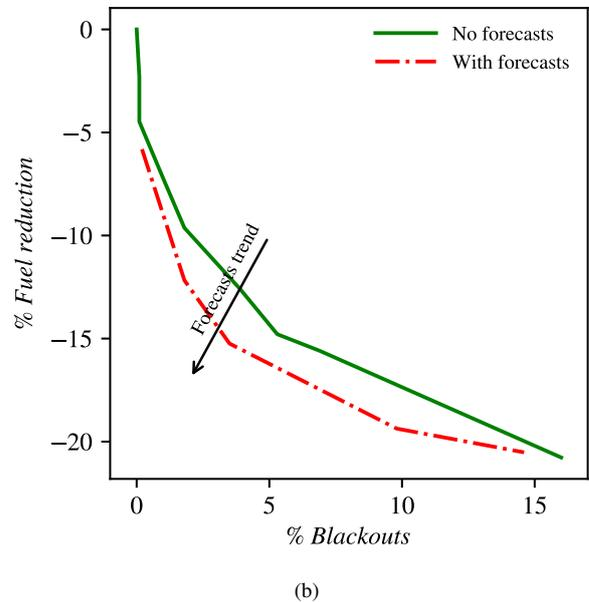
Fig. 4. Dependence of the percentage fuel reduction and percentage blackouts with the control criterion for: (a) the no forecasts approach, which varies as the control criterion  $\alpha$  and (b) the forecasts approach, which varies as the target percentile (%). For both cases, the control scheme goes from passive to very aggressive PV injection control scenarios (from left to right on the x-axis).
