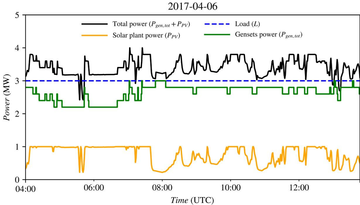
Fig. 3. Simulated power profiles of the system components on the 2017-04-06, with the gensets' control performed using the sky-imager forecasts. When the total power is below the load, a blackout occurs.
