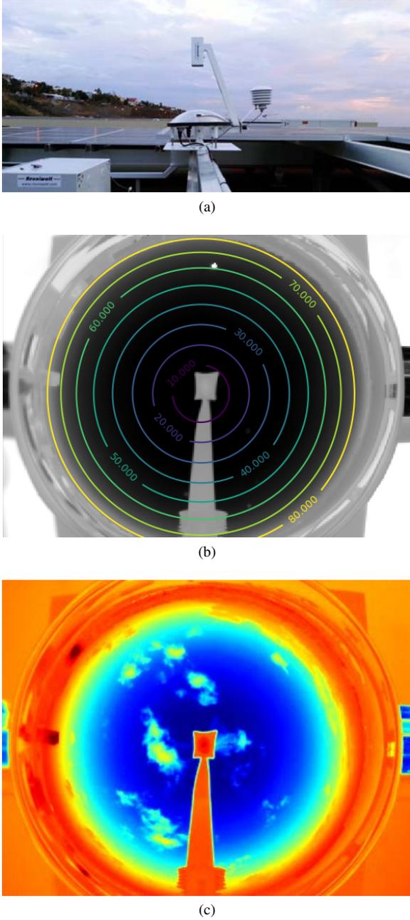
Fig. 2. (a) The Sky Insight thermal-infrared sky-imager system at the site Le Portail, (b) geometric calibration showing the zenithal angles on the image and (c) thermographic image with clouds showed as warmer patches superimposed on the cooler clear sky background.
