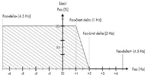
Figure 8. Frequency shift control for AC-coupling grid-tied inverters
