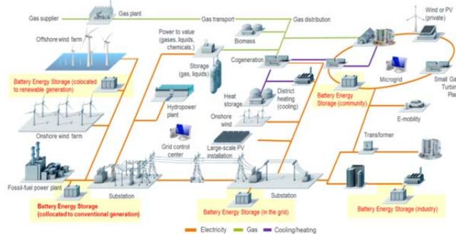
Figure 2: Integration of BESS in modern grid structures
