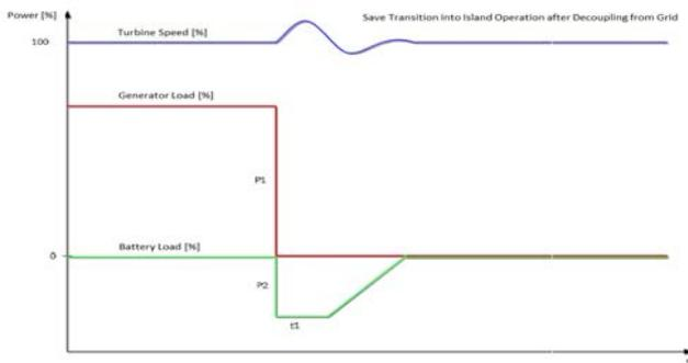
Figure 5: Turbine stabilization after disconnection from the grid
