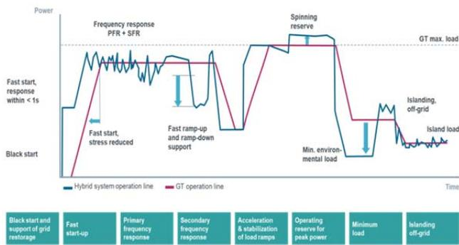
Figure 4: Optimized performance of hybrid system (BESS + GT)
