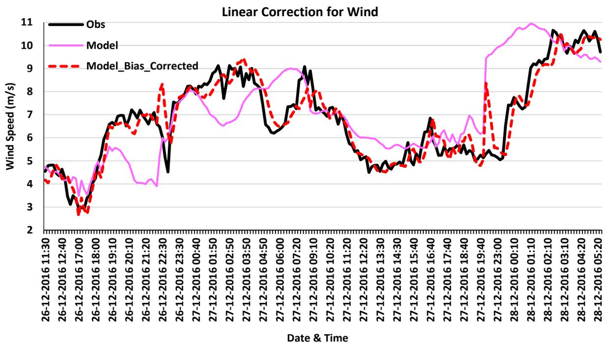
Figure 2. Time series of observed wind plotted with forecast using best model configuration (Pink color) and using linear bias correction (Red).
