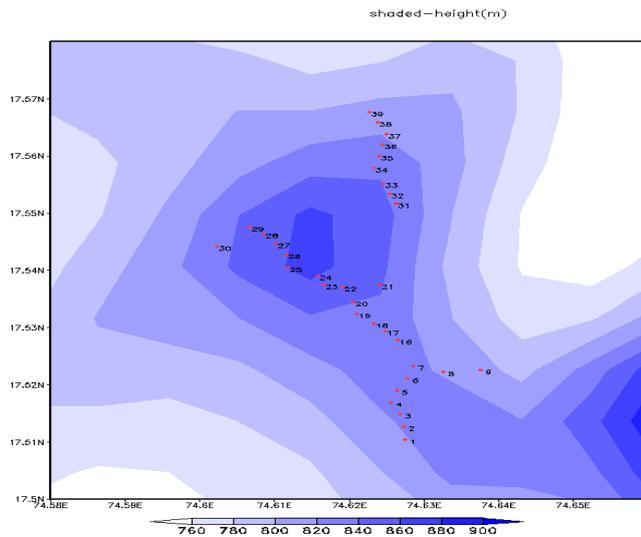
Figure 1b. Terrain Height in meter (shaded) at Agaswadi (Maharashtra state) wind Farm site in India. The dots represents the location of each wind turbine over the topographically complex site of Agaswadi. wind turbines are notes as T1-T9 and T16 to T39.
